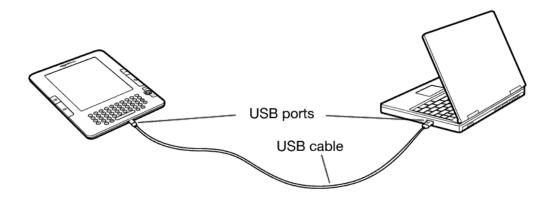
When you are connected to your PC, your Kindle will go into USB drive mode and its battery will be recharged by the computer. Your Whispernet service is temporarily shut off and you will not receive any of your subscriptions while in this mode. Also, your Kindle is not usable as a reading device while you are in USB drive mode, but will return right to where you were when you eject the device from your computer.
